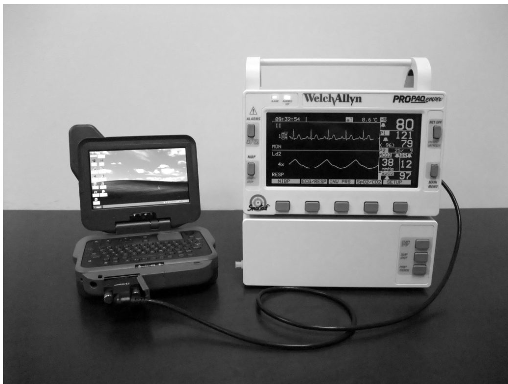
Fig. 1 Photograph of the Automated Processing of Physiologic Registry for Assessment of Injury Severity (AP-PRAISE) hardware components in the disassembled state. The GoBook MR-1 on the left is connected to the Propaq 206 on the right .
