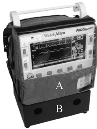
Fig. 1. Assembled prototype of the proposed system (under development in collaboration with Intelesense Technologies, Milpitas, CA). Propaq 206 vital-signs monitor “A” is mounted on top of the protective cage “B,” which contains the ruggedized Switchback PC.
