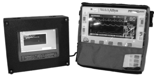
Fig. 2. Protective cage detached from the Propaq. LEFT: Bottom view of the cage, showing the touch screen of the ruggedized Switchback PC. RIGHT: Propaq 206 vital-signs monitor.
