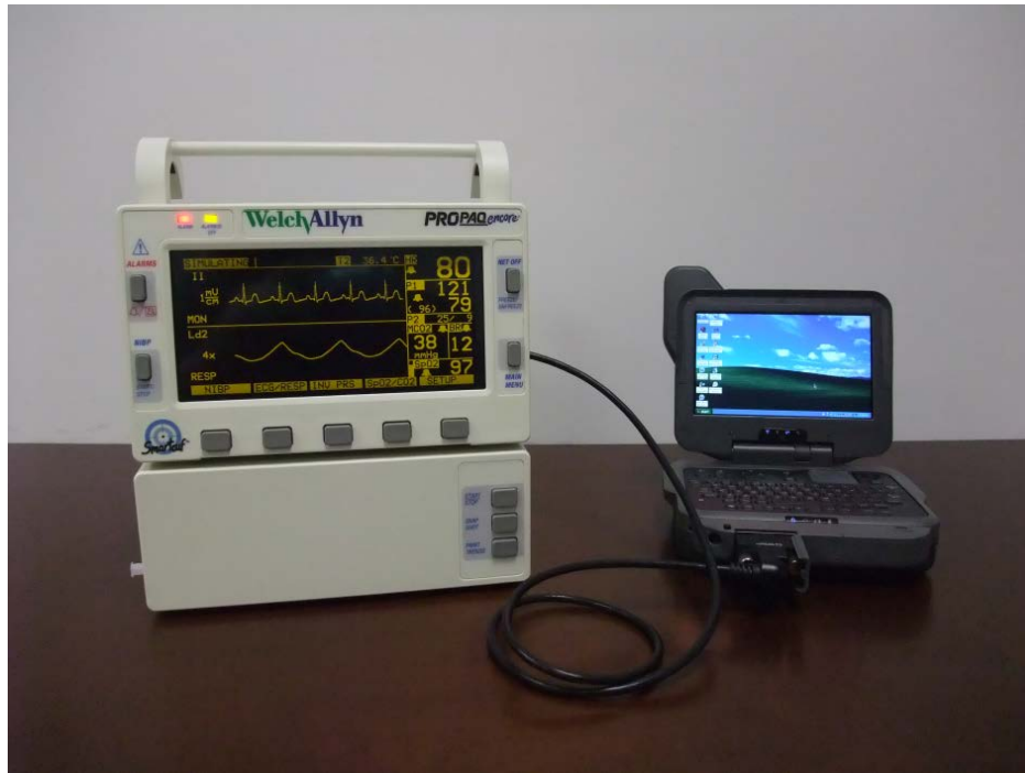
Figure 1: The hardware components of the APPRAISE system in a disassembled state. The GoBook personal computer (General Dynamics Itronix, Sunrise, FL) on the right is connected to the Propaq 206 patient monitor (Welch-Allyn, Beaverton, OR) on the left through an RS-232 serial cable. During field operations, the personal computer was affixed to the top surface of the Propaq monitor using nylon strapping and velcro (not pictured).
