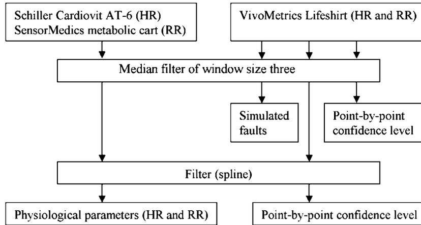
**Figure 1.** Datasets and processes used to develop and evaluate a fuzzy logic algorithm to assign confidence values to HR and RR.
